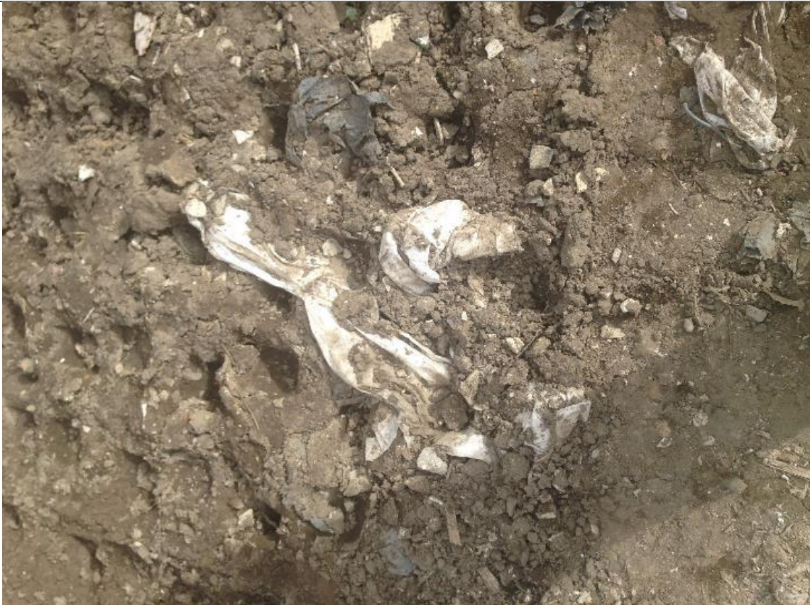
Photograph 2: An overview of the asbestos that was not adequately covered in the Asbestos Disposal Area. Note: Broken Asbestos fragments on the surface and evidence a compactor had driven over the area.
