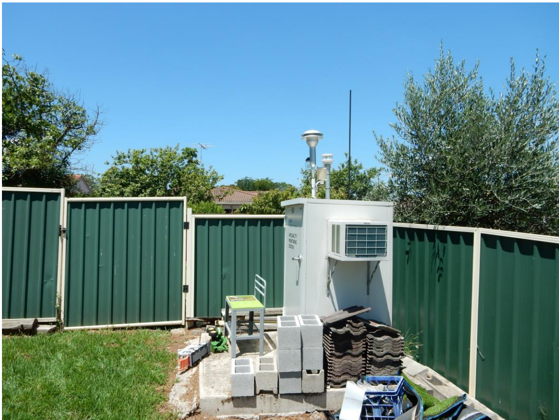
Photo 22: TEOM with tree covering the unrestricted airflow of the sampler inlet
