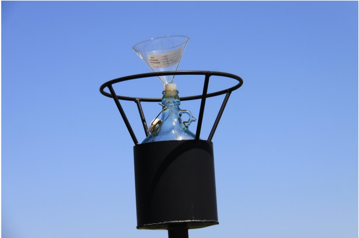
Photo 21: Dust gauge with funnel not horizontal and dust gauge not vertical.
