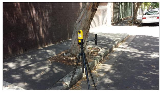
Photo 3.1 – Illustrated setup of the Kestrel Anemometer apparatus in operation (Source: The Odour Unit Pty Ltd)
