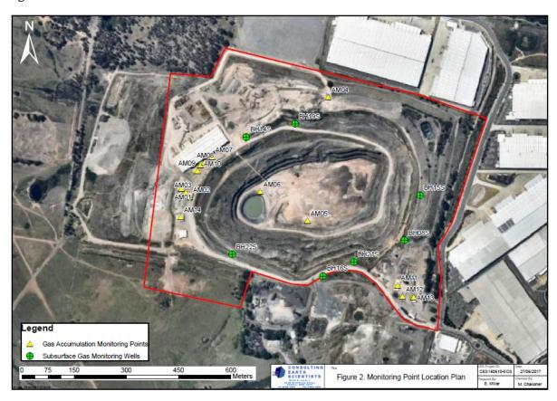
Figure 5-9: Landfill gas monitoring locations
