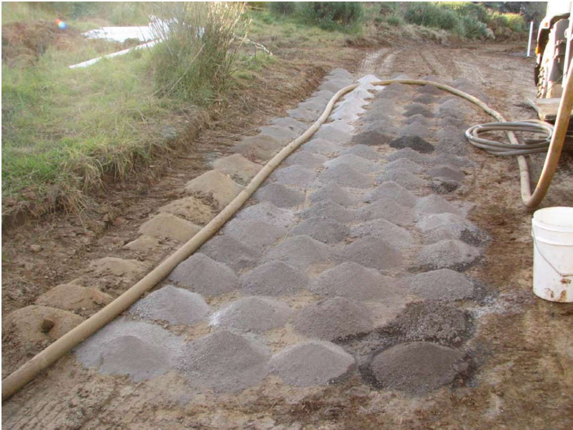
Drill cuttings from hammer drilling. Cuttings were collected on a metre basis and geologically logged for comparison with the core holes and to assess areas of groundwater inflow, together with the driller's observations.
