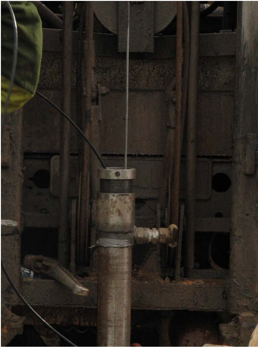
Packer setup with packer suspended by cable and the compressed air inflation hose passing through the fitting at the top of the rods. Water under pressure from the pump is supplied via the hose fitting on the right.
